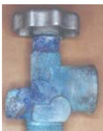
As observed in the illustrations, a blue-green stain on any brass portion of a service valve is evidence that it may have been in contact with anhydrous ammonia\*. The pungent odor of ammonia on or near the cylinder is also an indication. If you suspect that a propane cylinder contains or has contained anhydrous ammonia, exercise extreme caution and restrict access to the area.
