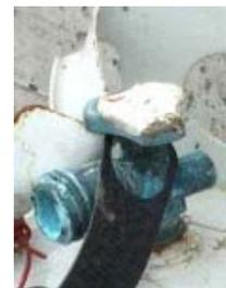
\*Note: Sherwood valves contain a green coated valve stem. Additionally, a green thread sealing compound is used on some valves. These valves should not be confused with those that have been exposed to anhydrous ammonia.
